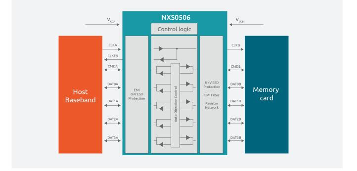
NXS0506 comes with auto-enable feature. If the supply voltage at Memory card side ( $V_{\rm CCB}$ ) rises above 1.5 V, the level translator logic is enabled automatically. As soon as  $V_{\rm CCB}$  drops below 0.65 V, the memory card side drivers and the level translator logic are disabled. The device features an auto correction control for all data channels except CLK.
